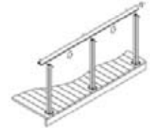
3-INSTALL TOP RAILS
