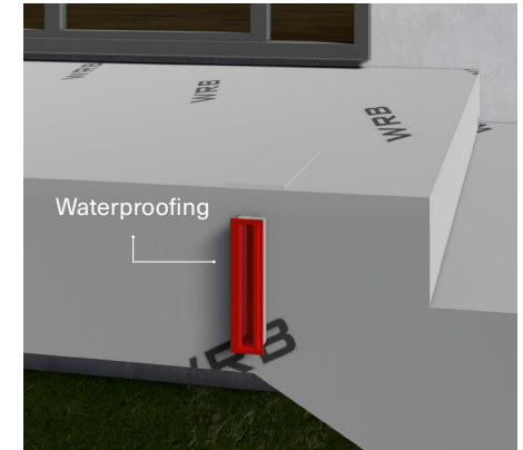
STEP 3 Waterproofing over mounting base plate
