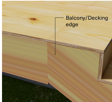
STEP 1 Complete balcony framework
