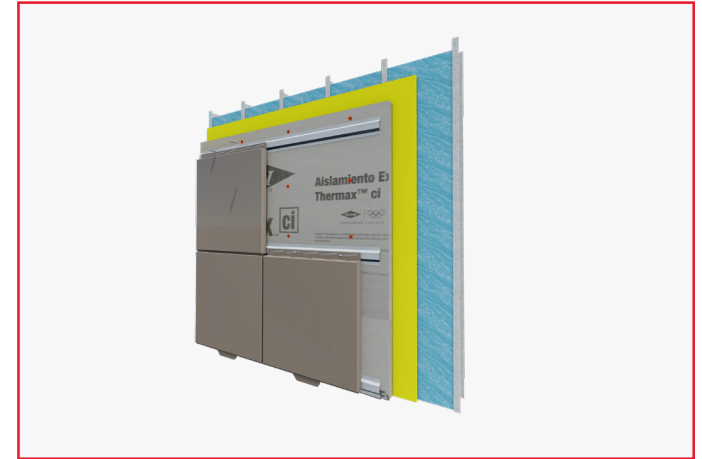
HAT CHANNEL OVER EXTERIOR INSTALLATION
