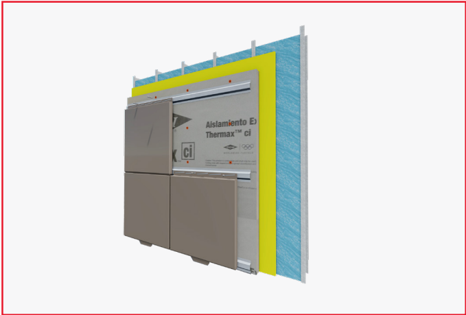
HAT CHANNEL OVER EXTERIOR INSTALLATION
