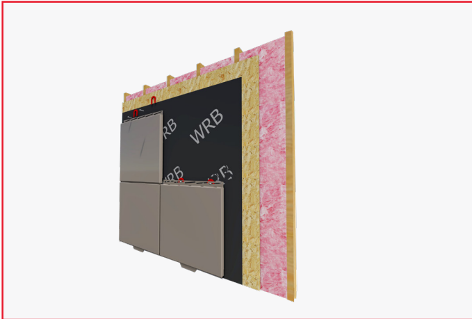
DIRECT MOUNT OVER WOOD FRAMING & SHEATHING
